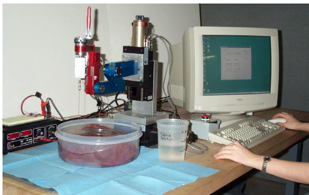
Figure 1. The data acquisition system was comprised of the JHU Steady Hand Robot, a needle holder with load cell, and a control computer.
